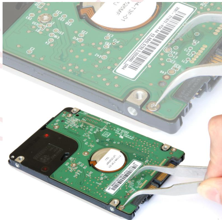
Fig.8.2. Another variant of insulator insertion.
